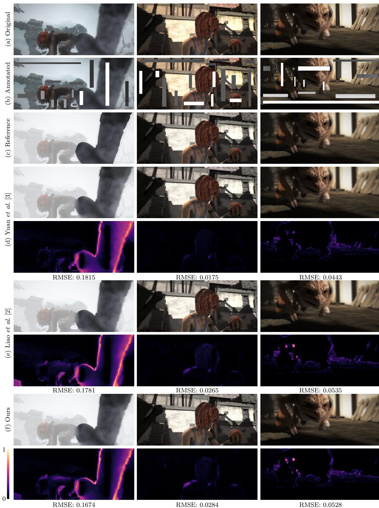
Fig. 4 A comparison between haze (left), desaturation (middle) and refocus (right) depth-based effects generated by related work (d, e) and our approach (f) for the Sintel dataset [1] (a) that we sparsely depth annotated (b). False color maps show perceptual differences to the reference images (c).
